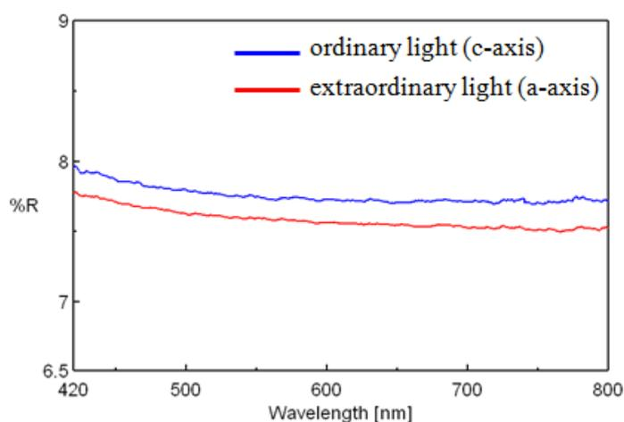
Fig. 1. Absolute reflectance spectra of monocrystalline sapphire
