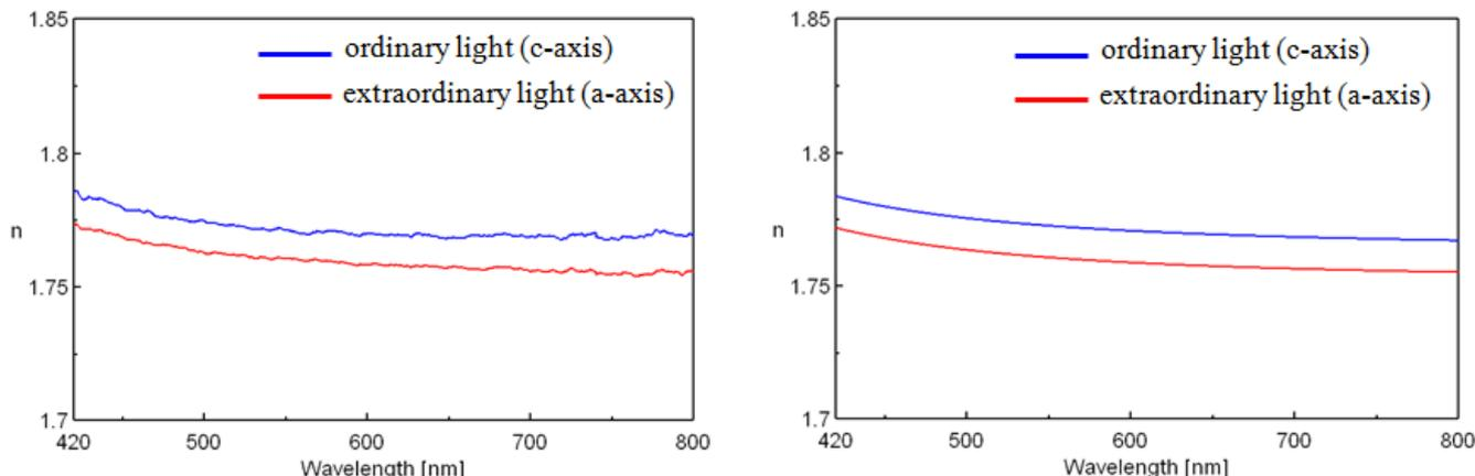
Fig. 2. Wavelength dispersion of refractive index of monocrystalline sapphire (left: left: by using [UV-Vis K-K Conversion] Program, right: by using [Multi-layer Analysis] Program)
