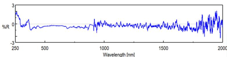
Fig. 4. Error between measured and calculated spectra
